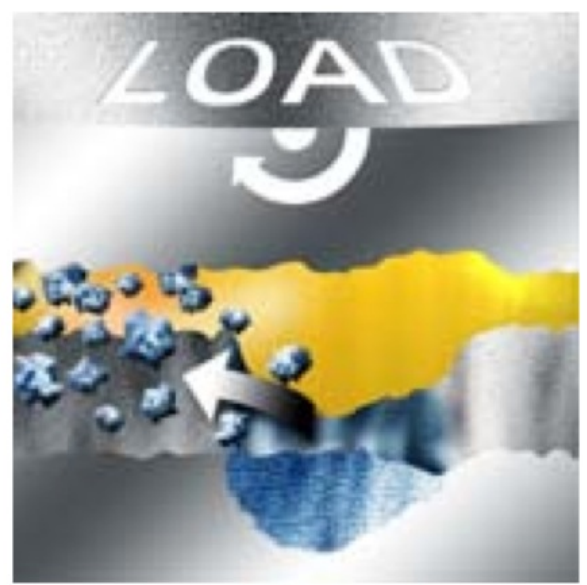
4. Surface fails + created particles
